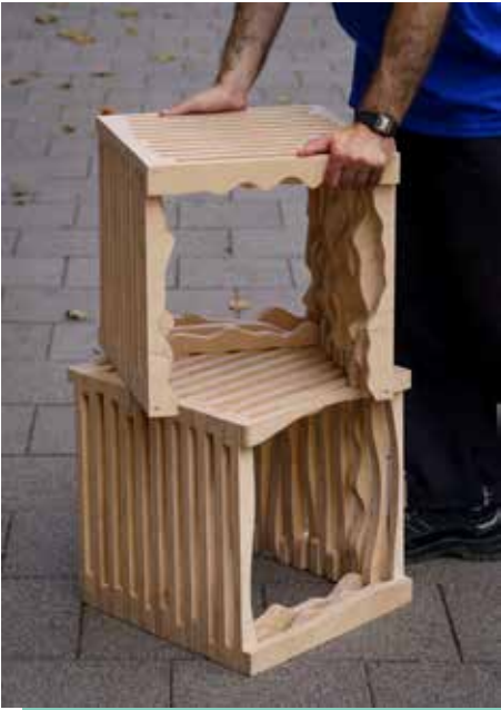
Artist Jesse Howard and SME Fiction Factory used software to dynamically create objects from left-over sheet material in CNC production, making shelving units, stools and wall cladding. Photo Iñigo Puerta Uranga
