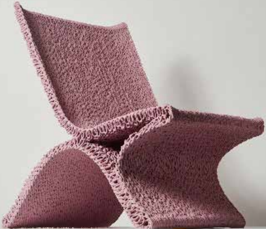
The result is printing in loops, rather than layers, seen here in the Loopy Chair - Photo by James Champion
